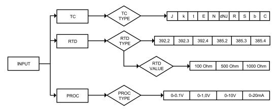
Figure 3.3 Flow Chart for Input Type Menu
